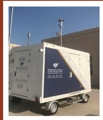
Mobile Air Quality Monitoring Station
