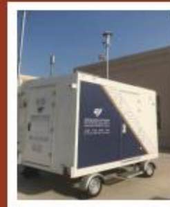
Mobile Air Quality Monitoring Station
